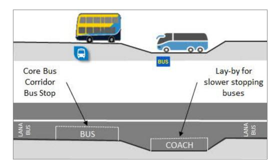
Figure 1.7 Double Bus Stop (in-line for BusConnects routes) concept for locations with buses requiring different dwell times.
