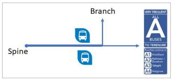
Figure 6.3 Location of Bus Stops Immediately before Branch Route Peels Off Spine
