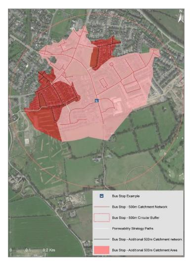
**Figure 4.1** Passenger catchment analysis for a bus stop indicating the existing and possible catchment areas assuming permeability improvements can be undertaken.
